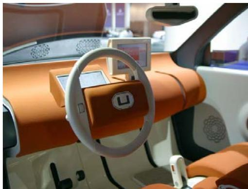
Figure 1: Picture showing the actual vehicle interior with the GUI display mounted on the dashboard.
